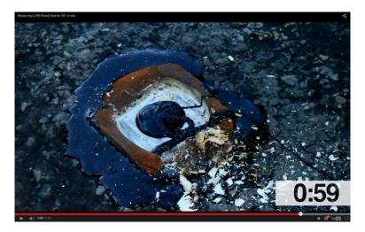
5. Place a new 290 reflector into the 301 casting, pressing gently into place, ensuring that no adhesive covers the reflector lens.
